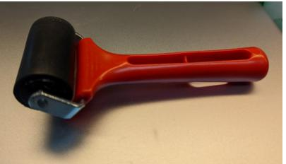
We recommend an ink roller like this that has enough flex in the rubber to be able to push the foil into each well to get a fully concave, tight seal
